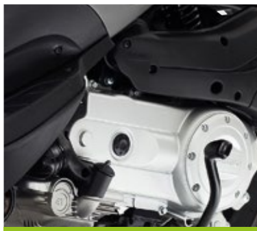
NEW 50 CC I-GET ENGINE 4-STROKE, 3 VALVE ELECTRONIC INJECTION EURO 4
